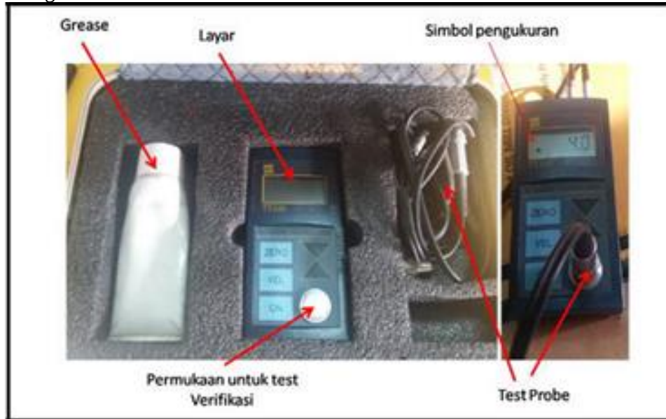
Gambar 1. Smart Sensor Ultrasonic Thickness Gauge TT 130
