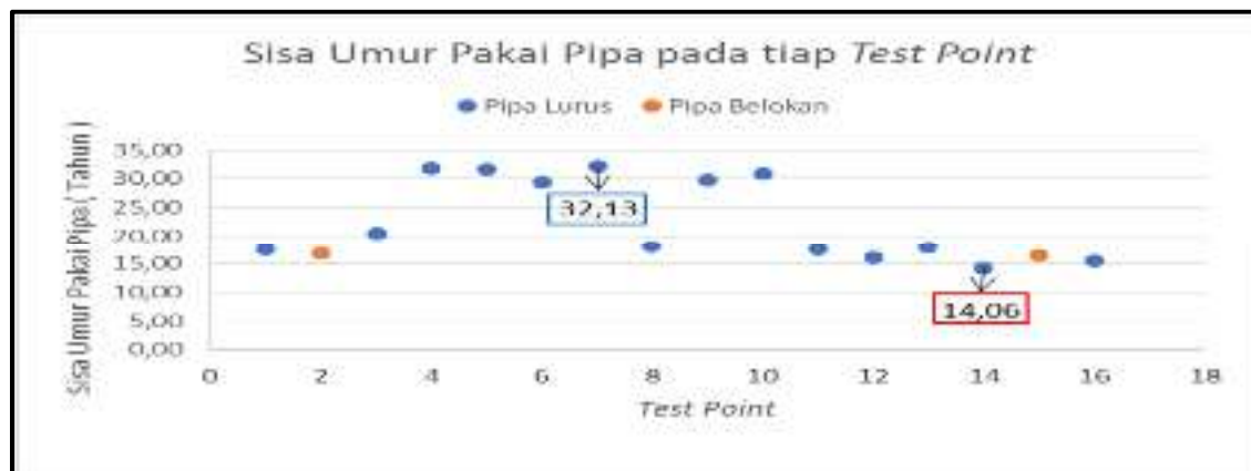
Gambar 1.4 Sisa Umur Pakai Pipa Transportasi Gas
