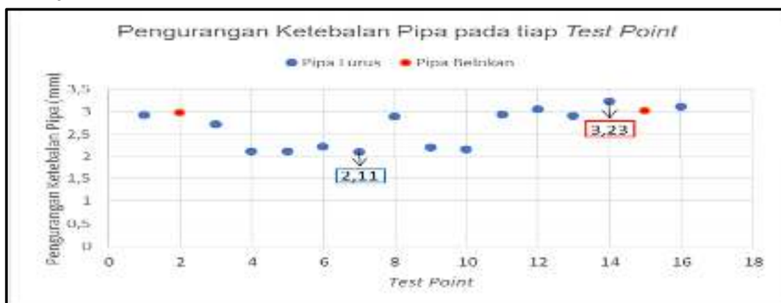
Gambar 1.1 Pengurangan ketebalan Pipa Transportasi Gas
