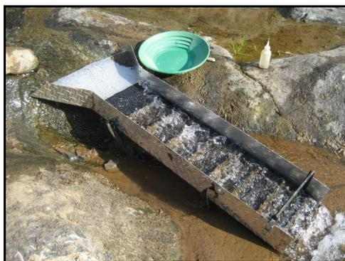
**Gambar 1.** *Sluice box* Aluminium
